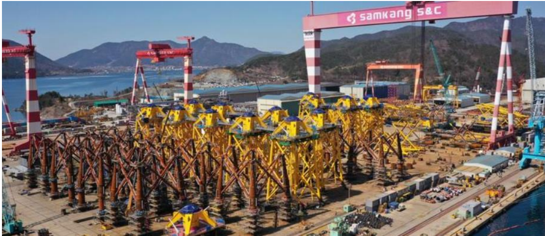
Figure 4-4: Jacket foundation manufacturing at Samkang Shipyard, Korea [6]
