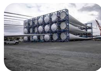
Storing blades in stacks of three
