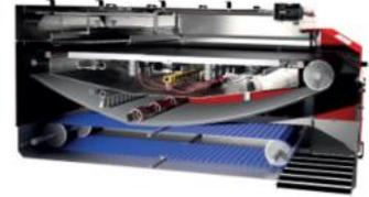
difference is that the ModCube combines a high air flow through a rotating filterbelt with microvibration compared to the vibrating screen of a shaker.
