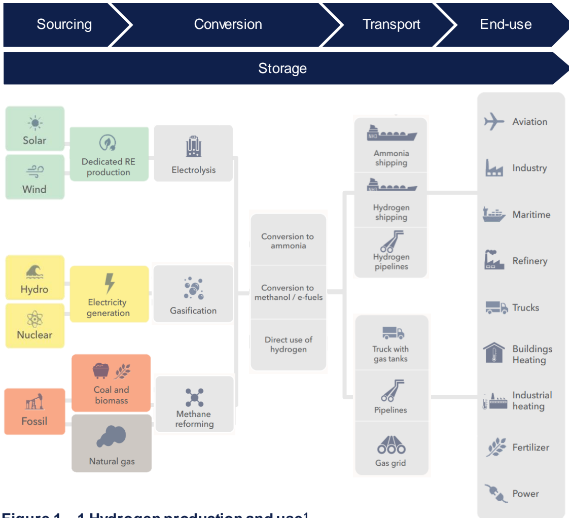
Figure 1 – 1 Hydrogen production and use 1
